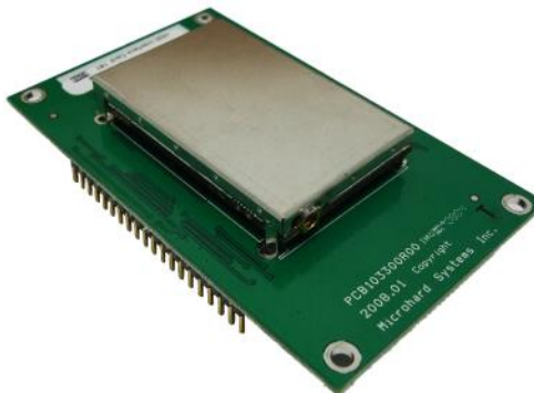
Image 3-4: Nano Interface Card with n920 Installed
